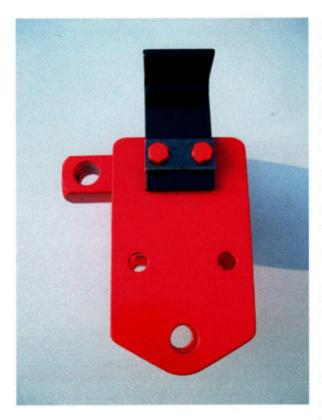
Bolt the slotted "L" shaped push bar using the provided 3/8" X 3/4" grade 5 hex bolts and the small 1/8" thick 2-hole tie plate to the lower side of the Weldment into the 2 tapped hole with the "L" facing down, away from the horn receiver block of the Weldment. Apply a little oil or light grease before inserting bolts into threads. Leave these bolts snug till final adjustment to your machine. The 2-hole tie plate provides a better locking grip for the push plate than simple washers.
