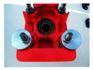
The provide "U" shaped 2 hole push plate (also called 2-stud reinforcement retainer plate) is attached to the lower two double ended Q H studs (not supplied with this kit) of your quick hitch. The optional "horseshoe" shaped 4-stud reinforcement retainer plate
