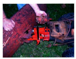
To attach your old dozer blade, first remove the 4-bolt advance casting mounting adapter blade support from the blade swivel casting. You will not need that adapter for this assembly. Slide the new quick hitch adapter into the blade swivel casting and drop in the new supplied
