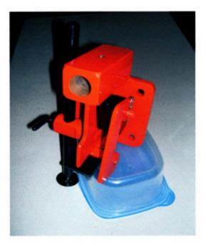
At the time of this printing, Cogan Valley Machine Co. has produced a "Quick Hitch Non-Powered Attachment Adapter" for use of attachments such as the tool bar, wheel barrow, or dump scoop with the Gravely quick hitch system. This adapter was developed to attach a custom built two wheeled cart to the quick hitch, but could be used with nearly any Gravely built 4-bolt mounted attachment with a flat mounting surface.
