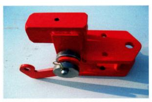
At your option, install the 1/2" threaded shoulder pin through the provided 3/8" hole located on the opposite side from the drop leg lug for storage of the accessory hardware (secured with the smaller hair pin through a hole at the end of
