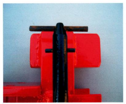
The drop leg of your adapter needs to be assembled in place. 2 roll pins are provided to install through the upper 2 holes of your drop leg. The long pin (1/4" X 3") acts as a handle, the shorter (3/16" X 1-1/2"), when installed, provides
