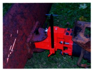
With the use of the drop leg, disconnecting from your walk behind tractor is simple and easy. When in use, the drop leg is stored by raising it up through the drop leg lug and locked with the "L" shaped clamp bolt handle. The supplied hairpin can be slipped
